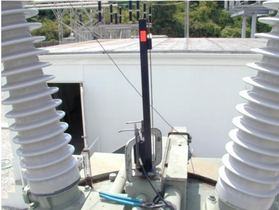
Linear Transducer on an OCB
